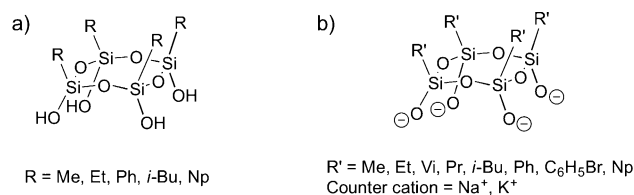
Figure 2. Suggested structures of a) the [RSiO(OH)]_4 half-cube; b) the [R'SiO(OM)]_4 half-cube salt.
